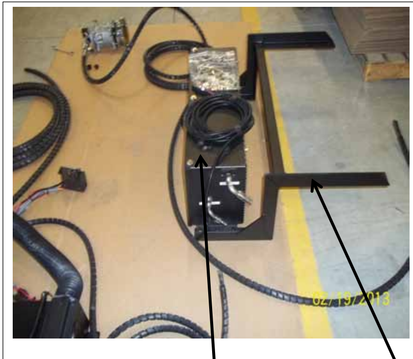
Condenser with drier mounted inside the box.
