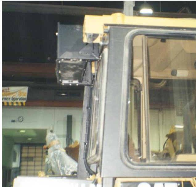
Condenser assembly viewed from side.
