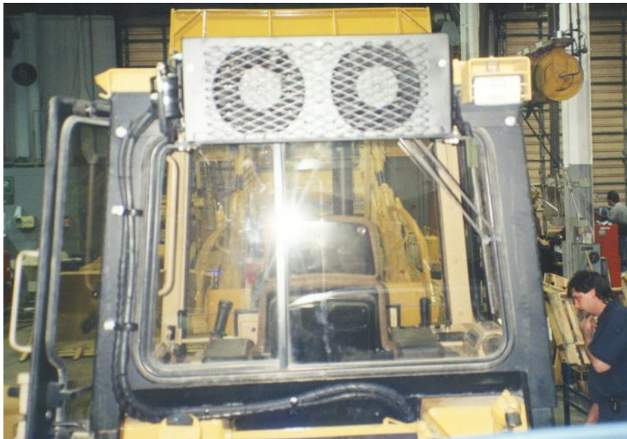
Condenser assembly viewed from back of machine.
