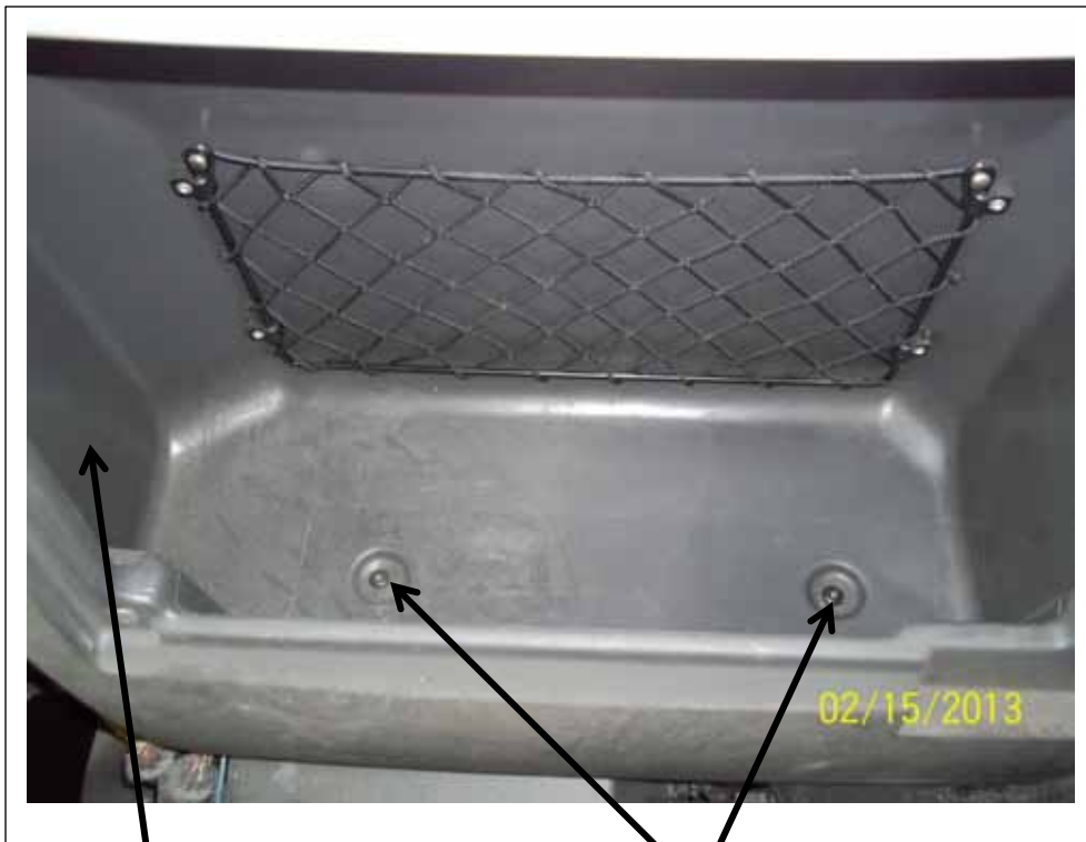
Remove these two screws and discard. Lower evaporator bolts will fasten here.
